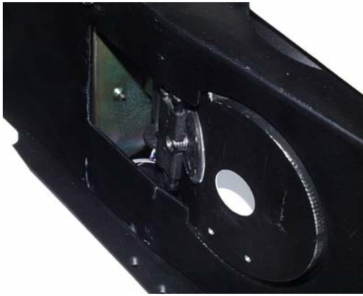
The specular exclusion port closed (RSIN mode)
