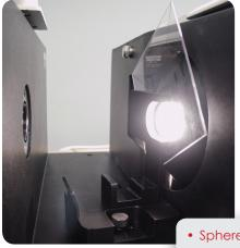
The ColorQuest® XE offers an excellent value The efficient optical configuration delivers high performance with a true monochromator design. Sealed dual beam optics incorporates a diode array detector that allows simultaneous measurement of the sample with real-time reference beam
