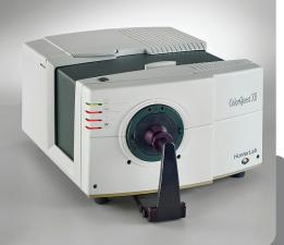
Using d/8° sphere geometry, the rugged, dependable ColorQuest® XE measures opaque, transparent, and translucent solids and liquids, offering exceptional price-performance value. In the lab or on the production floor, the versatile ColorQuest® XE measures a variety of color values, in every viable color scale in the 400 nm - 700 nm spectrum.
