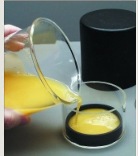
Orange juice sample being prepared for measurement using a “Ring and Disk” assembly.
