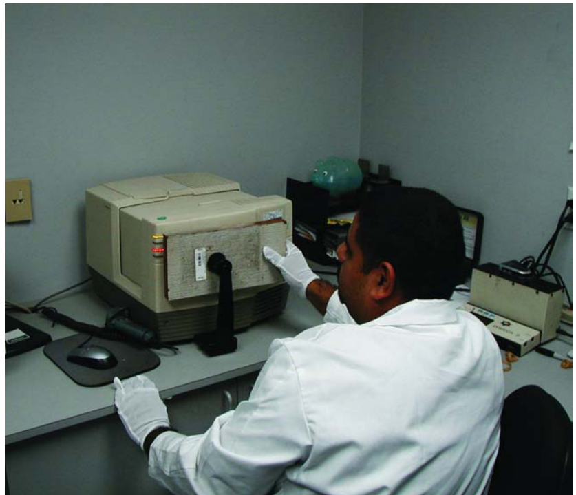
An evaluation technician measures color change on painted wood test panels in a special environmentally controlled laboratory. Photo courtesy of South Florida Test Service.
