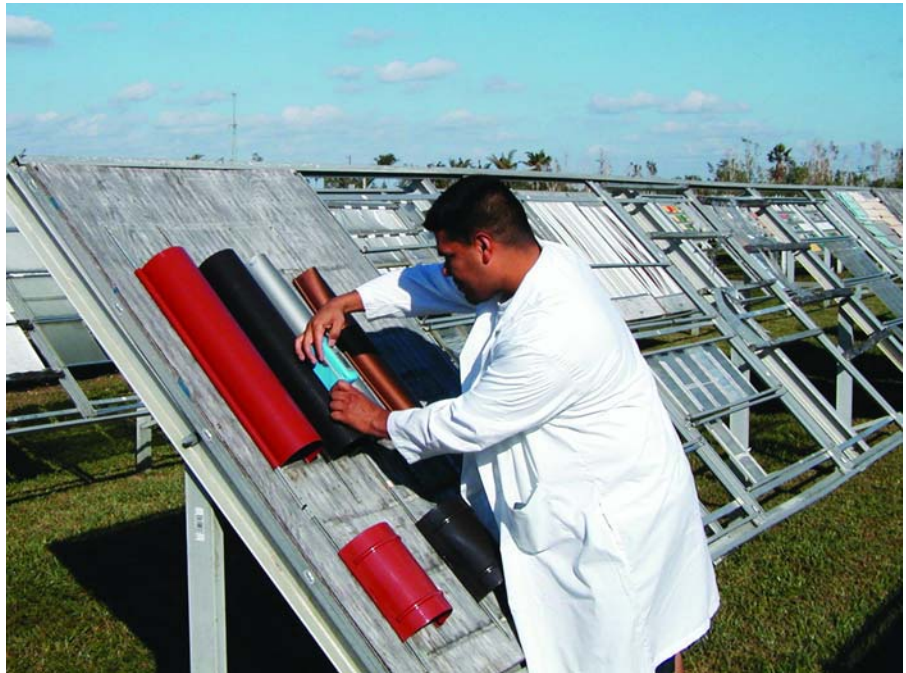
Gloss measurement being performed on a weathered architectural detail too large for in-laboratory measurement. Photo courtesy of South Florida Test Service
