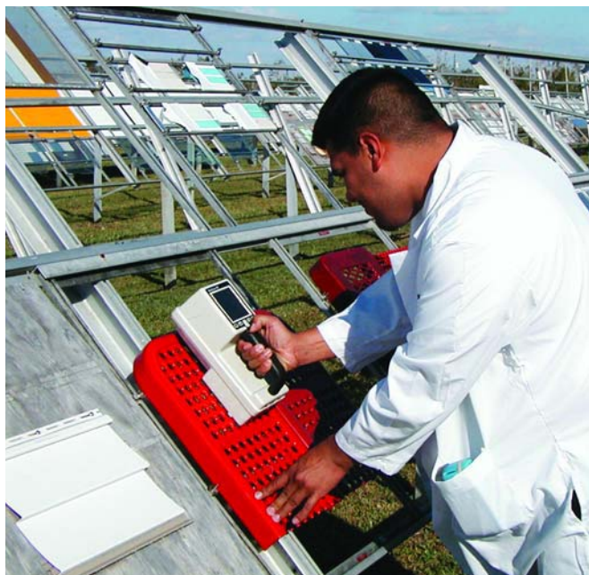
A weathering laboratory technician performs a field measurement on an architectural detail for color change. Photo courtesy of South Florida Test Service.
