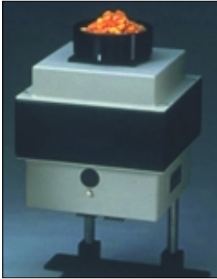
HunterLab D25L Tristimulus Colorimeter sensor shown with snack food sample.
