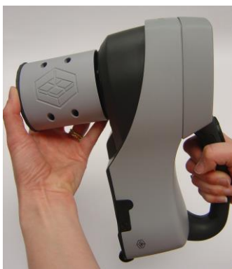
Figure 16. Reading the Calibration Cylinder
