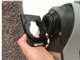
Figure 26. Inserting the Nose Cone Adapter
