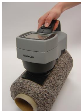
Figure 27. Using the Nose Cone Adapter
