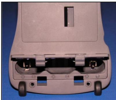
Figure 3. Battery Compartment of the MiniScan EZ
