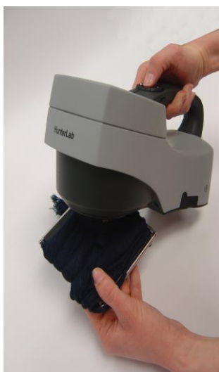
Figure 29. Measuring with the Skein Holder
