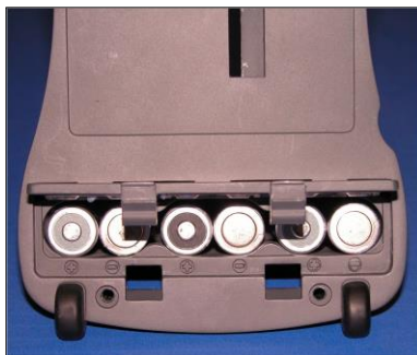
Figure 4. Install AA Batteries
