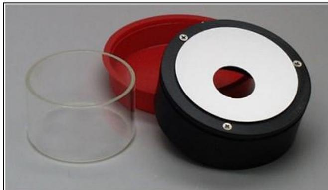
*Figure 59. Modified Port Insert, Cap and Sample Cup*
