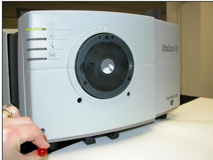
Figure 53. Front Cover Screws
