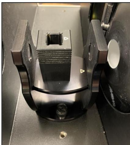
*Figure 74. Cell Holder Installed*
