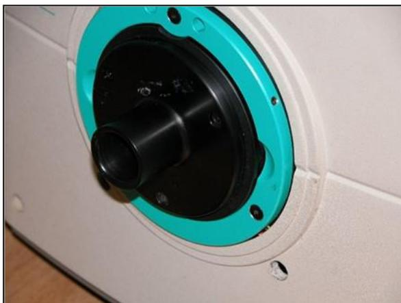
Figure 78. Insert Port Plate
