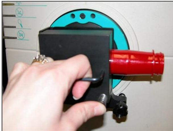
*Figure 68. Preform Holder Installed*
