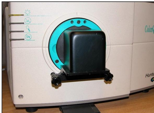
*Figure 71. Light Cover over Sample Container*
