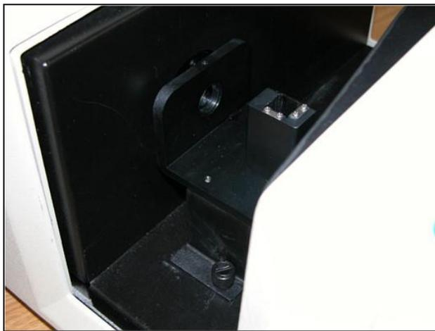
Figure 76. Insert Cell Holder
