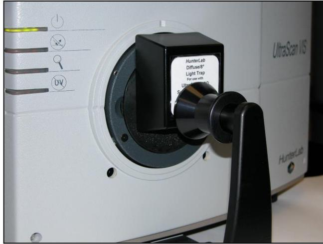
*Figure 21. Standardizing with the Light Trap*
