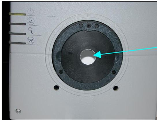
The reflectance port with the large area view port plate installed
