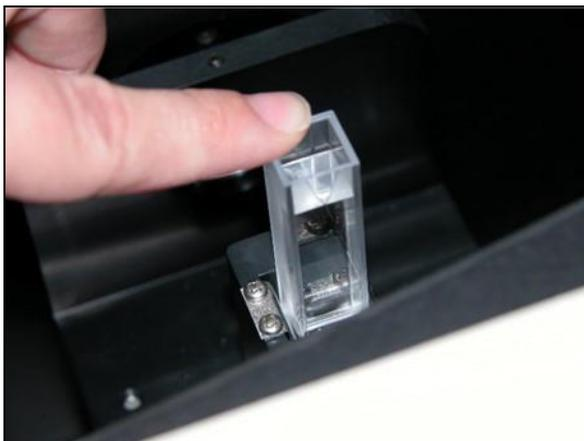
Figure 77. Insert Cell in Holder
