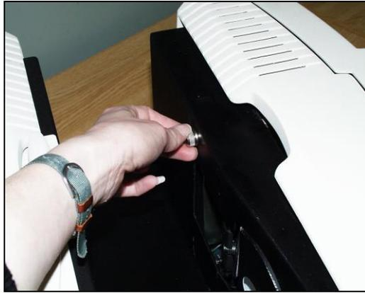
*Figure 54. Inside Cover Screws*
