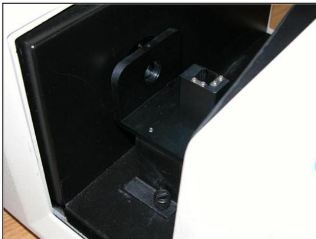
Figure 76. Insert Cell Holder
