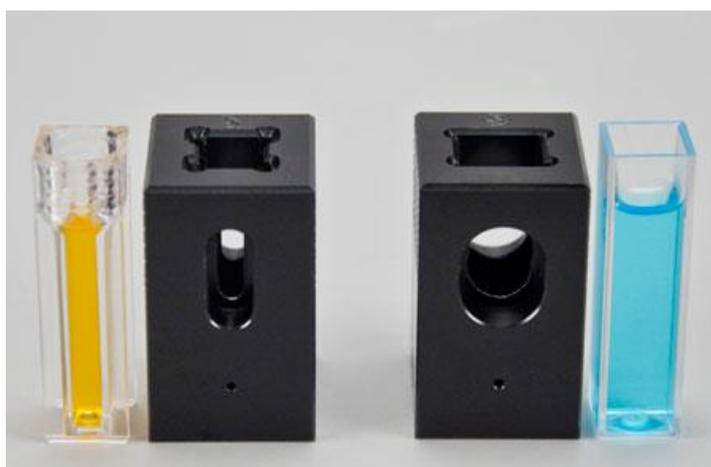
*Figure 75. Typical Semi-Micro Cell and Macro Cell Holder*
