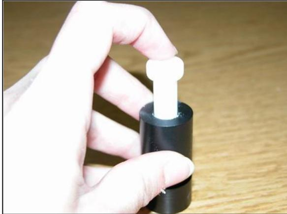
*Figure 79. Pack the Powder with the Plunger*
