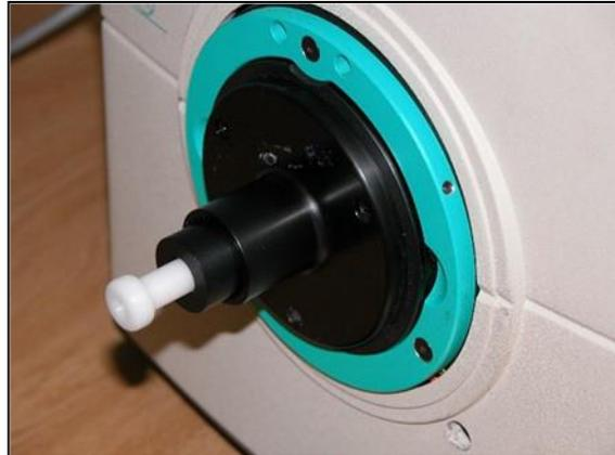
*Figure 80. Insert Powder Holder in Port Plate*
