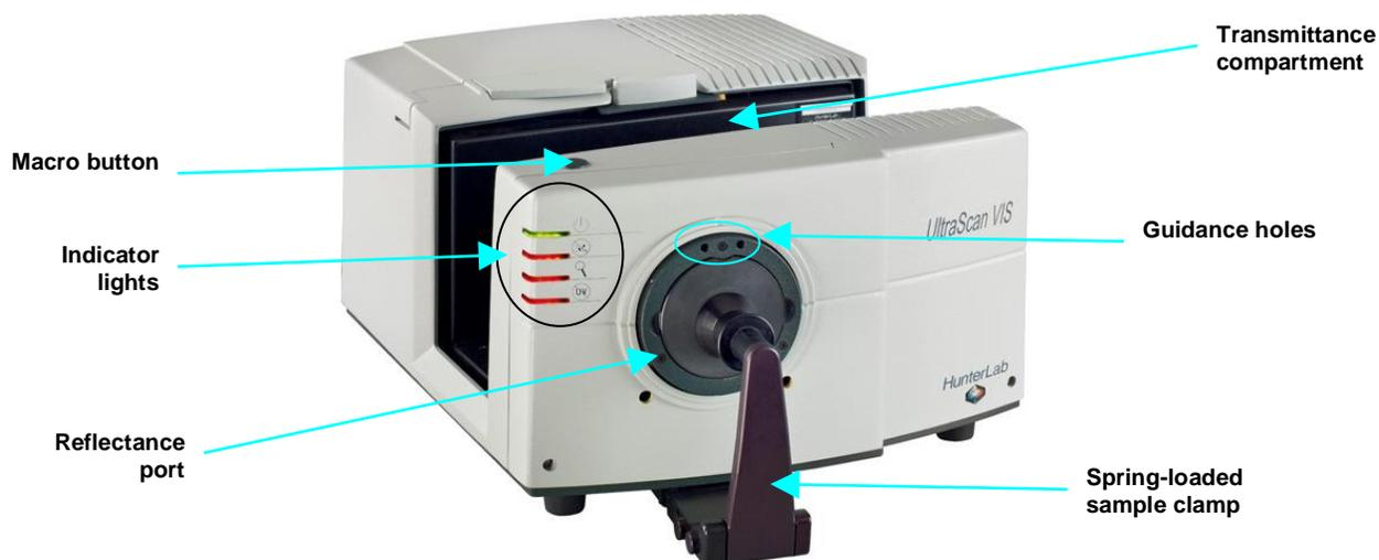
Figure 1. UltraScan VIS
