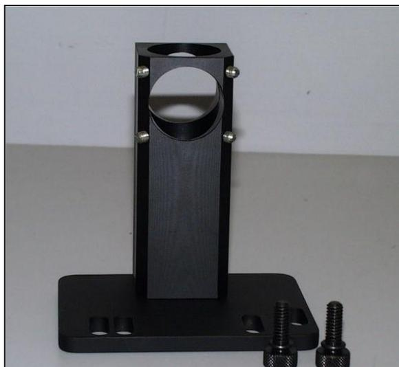
*Figure 61. Cylindrical Cell Holder*
