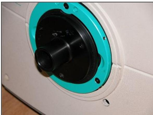
Figure 78. Insert Port Plate
