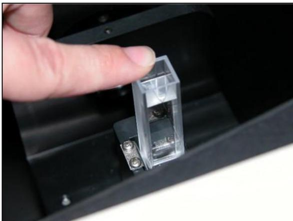
Figure 77. Insert Cell in Holder
