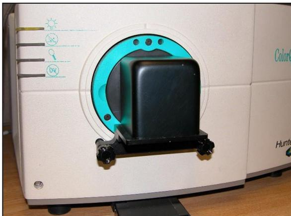
*Figure 71. Light Cover over Sample Container*
