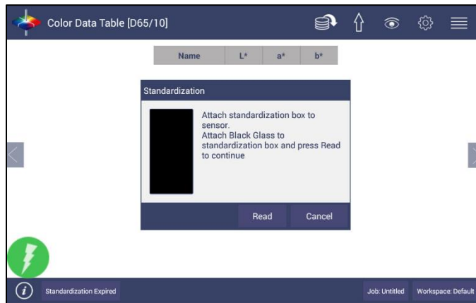
Figure 6. Read the Black Glass for Bottom-of-Scale
