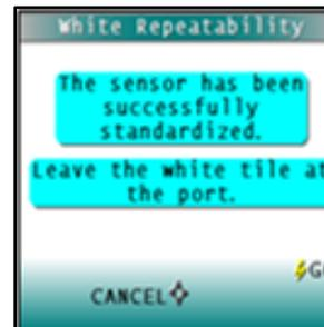
normal standardization for the instrument. When standardization is complete, the user is then prompted to leave the instrument white tile in position at the sample port and to press the **GO** button.
