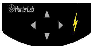
The five buttons on the button pad can be loosely defined as the **LEFT**, **RIGHT**, **UP**, and **DOWN** buttons, with the “**GO**” (lightning bolt) button located to the right of the arrows. These buttons perform slightly different functions based on the current operation. Consult the miniature map of the button pad shown at the bottom of the LCD display for the relevant definitions of the buttons at any particular time.
