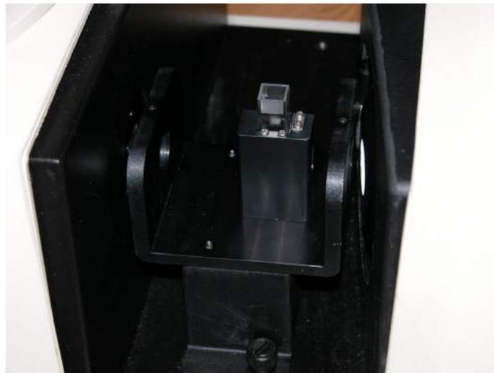
6. Complete the standardization by measuring the cell blank as the top of scale.
