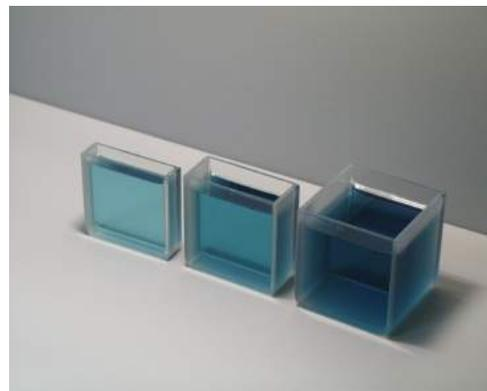
For transmission measurements, use the cell size recommended by your measurement specification (such as an ASTM method), or use the general rule that smaller path lengths should be used for more concentrated colorants.
