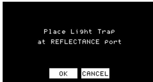
9. Mount the light trap at the reflectance port as instructed and either touch **OK** or press the Macro/Read button on the instrument. The ColorQuest XE reads and then the following prompt appears.
