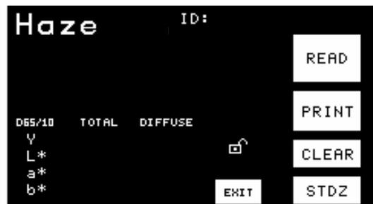
5. Touch **Stdz** to standardize the instrument in TTRAN mode by following the on-screen prompts. Note that there is an extra prompt for mounting and reading the light trap.
