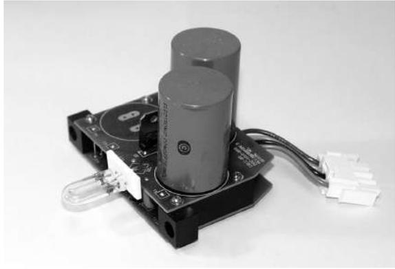
Before you attempt to change the source lamp, ensure that the UV filter is out. If the UV filter is left in, the filter may be broken during the process of removing and re-inserting the bezel. Check the UV Excluded indicator light. If the indicator light is on, you must restandardize the sensor in a mode with the UV filter out. (The filter can also be manually removed from the path, if necessary, by a trained representative of HunterLab.)
