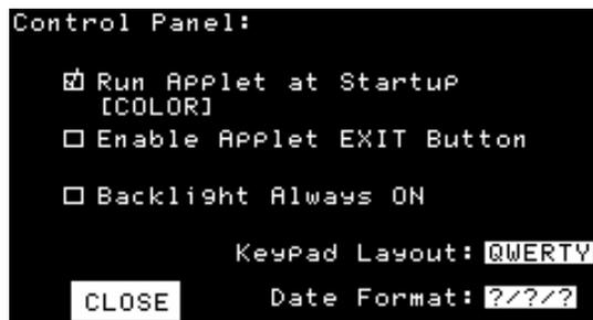
If you wish for users to be able to use the **Exit** button to leave applets even when they are locked, touch the box next to "Enable Applet EXIT Button" so that it is checked.
