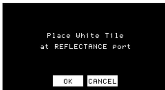
10. Mount the white tile at the reflectance port as instructed and either touch **OK** or press the Macro/Read button on the instrument. The ColorQuest XE reads and then returns you to your measurement screen. Standardization is complete.
