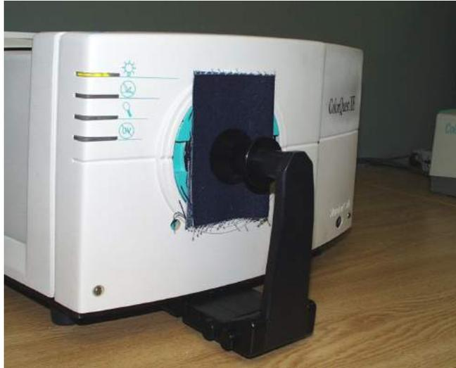
**The ColorQuest XE measuring a textile sample in reflectance**
