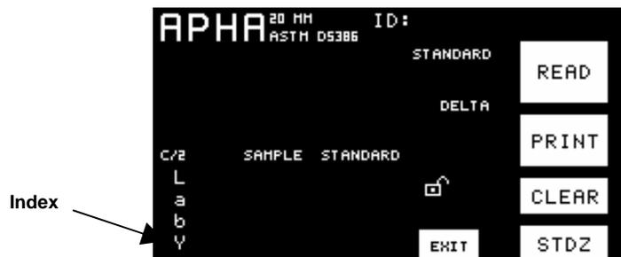
6. Touch the index area (which says “Y” in the screen shown above) until YI is shown. You may be required to touch and release the index multiple times before YI is displayed.
