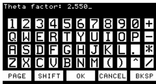
When you touch **OK** after entering the Theta factor, the measurement screen then shows Saybolt\*, indicating that the Saybolt factors have been optimized. Measure Saybolt as you ordinarily would.
