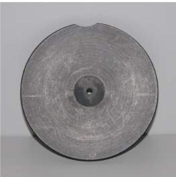
This option provides a modified port plate with a 4-mm round opening. This port plate should only be used when the small area view option is available and in use. To install the port plate, remove the standard port plate and snap the modified port plate into place at the reflectance port. Standardize the instrument in a reflectance mode using small area view.
