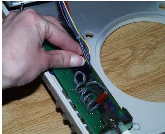
7. Remove the view lamp assembly and replace it with a new one. Be sure not to touch the bulb of the lamp as fingerprints reduce lamp efficiency. If a fingerprint is deposited, remove it using a clean wipe and isopropyl alcohol.
