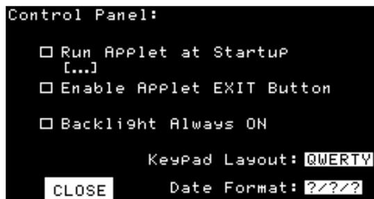
If you wish to begin running a specific Applet automatically whenever the ColorQuest XE is turned on, touch the box next to Run Applet at Startup so that the box is checked.
