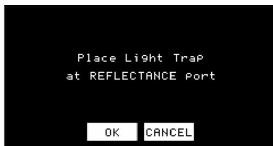
Touch **OK** to measure the sample with black at the reflectance port and display the diffuse transmittance and haze values.
