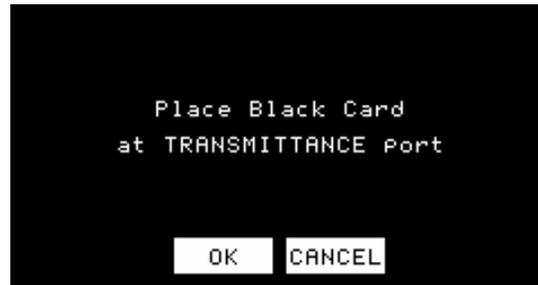
9. If you wish to standardize in TTRAN mode, place the black card flat against the transmission port (hole in the **sphere**). If you wish to standardize in RTRAN mode, place the black card flat against the **lens**. Then touch **OK** or press the Macro/Read button on the instrument. The ColorQuest XE reads and then the following prompt appears:
