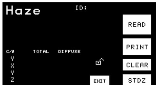
First, standardize the instrument in TTRAN mode by touching **Stdz** and following the on-screen prompts. In the haze applet only, a third prompt is added to the standardization process as shown below. It requires you to mount the light trap at the reflectance port.
