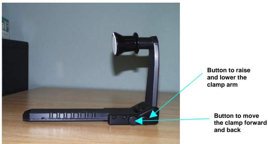
A magnetic white ceramic disk on the face of the clamp provides a consistent white background for measurements. A non-slip black pad (also magnetic) is also included that can be used to replace the white disk for applications that require a non-slip or dark backing. To change to the pad, simply pop out the white disk and insert the non-slip pad.
