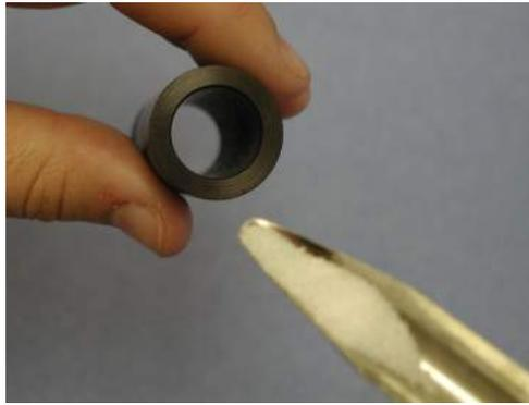
4. Pack the powder down using the plunger. Do not overtighten the powder holder. The powder should be at least 1/2-cm deep in the holder.
