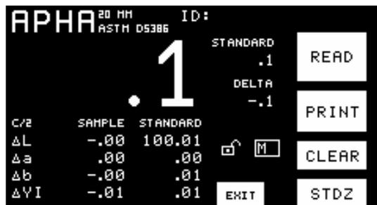
*Note: The instrument flashes three times for each APHA measurement because of the sensitivity required.*
