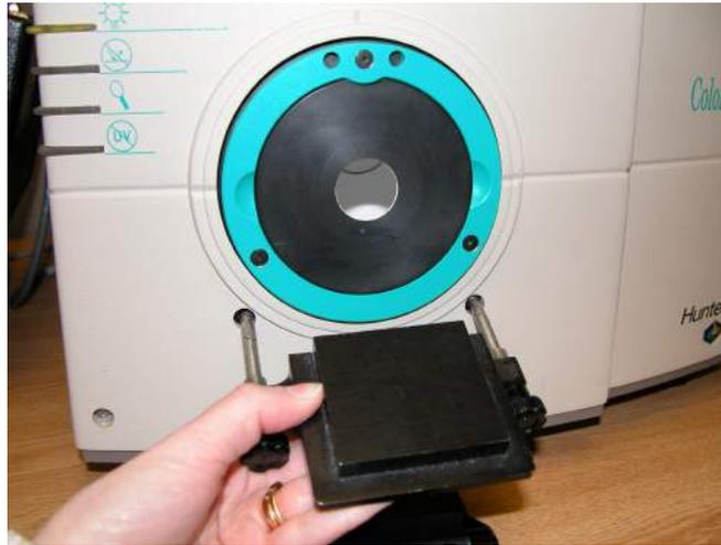
3. Tighten the sample shelf into place by turning both knobs clockwise.
