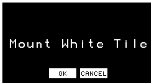
4. Mount the instrument white tile at the reflectance port and then touch **OK**. The ColorQuest XE reads and then the following prompt appears.
