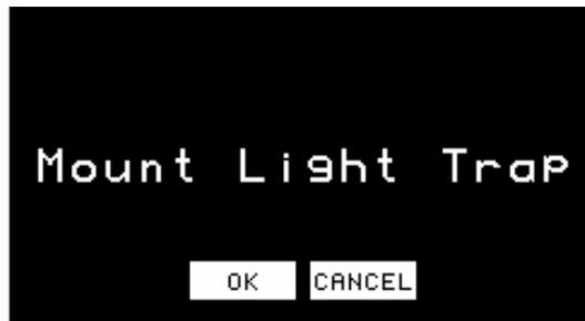
3. Mount the light trap at the reflectance port and then touch **OK**. The ColorQuest XE reads and then the following prompt appears.
