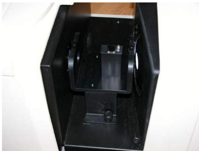
3. Initiate standardization in TTRAN mode for LAV, sliding the black card device between the cell holder and the hole in the sphere when prompted for the black card.
