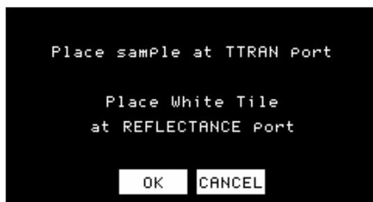
Touch **OK** to measure the sample with white at the reflectance port and display the total transmittance value.
