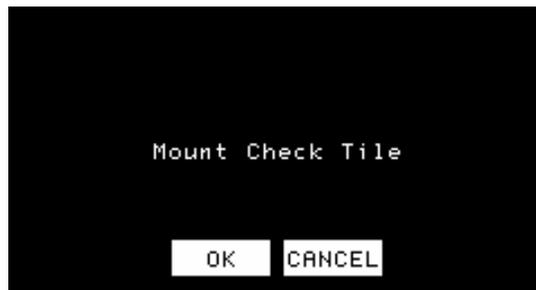
Five readings of the green tile are made and then you are prompted to remove the green tile and touch **OK**.
