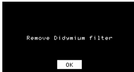
After the filter is removed and you touch **OK**, the end result for the wavelength test is shown.
