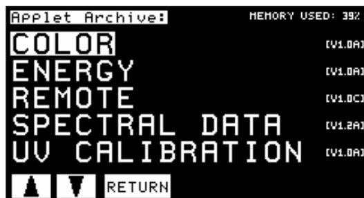
2. Touch the name of the applet you wish to load. (You may need to use one of the arrow keys to find the applet in the list.) The chosen applet is loaded into memory and available for use. When you touch **Return**, you will see that its name is added to the Select an Applet screen.
