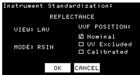
4. Touch the area just below “Instrument Standardization:” (where it says “Reflectance” in the example above) until “Reflectance” appears. Touching this area toggles you between Reflectance and Transmittance.
