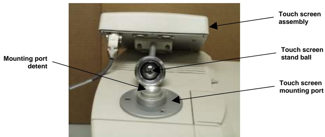
5. Standing in front of the instrument or on its left side, hold the touch screen assembly so that the screen is facing you and place the ball of the touch screen's stand into the detent in the mounting port.
