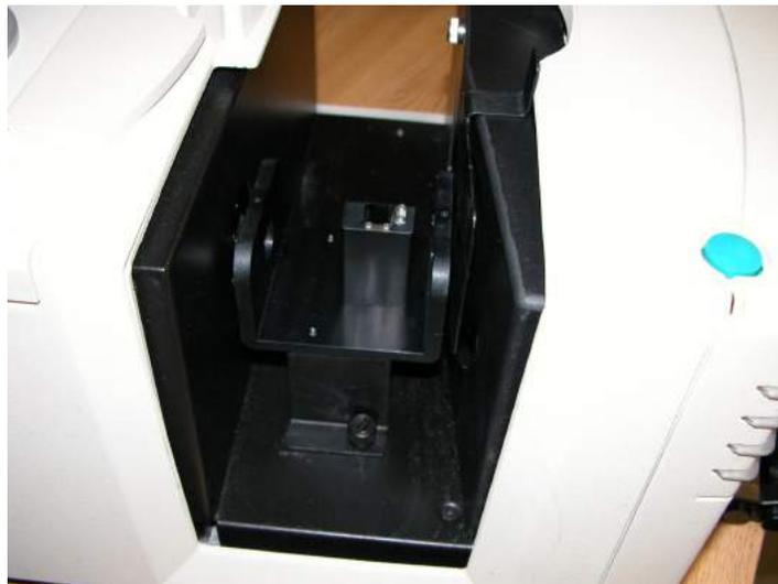
4. When prompted for the cell blank, fill the desired analytical cell with distilled water or another clear liquid you would like to use as your top of scale. Some cells will have a fill line. The liquid should at least reach this line.
