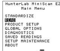
2. Press the **UP/DOWN** arrow to select a setup from the list. Press **GO** to continue.
