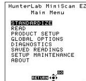
2. Remove the end cap of the calibration cylinder that covers the black glass (or light trap). Press the nose cone flush againsts the standard. Press **GO** to read.
