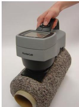
*Figure 83. Using the Nose Cone Adapter*
