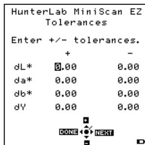
Change the highlighted digit of the selected color scale tolerance value using the **UP** and **DOWN ARROW** buttons. When the desired digit is shown, press **NEXT** to move to the next digit. Press **DONE** to return to the product setup configuration screen.
