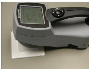
*Figure 66. Using a White Tile Backing*
