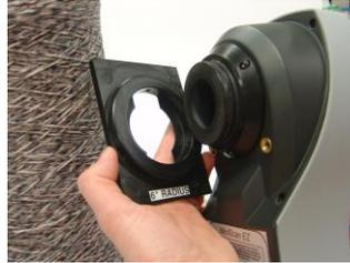
*Figure 82. Inserting the Nose Cone Adapter*
