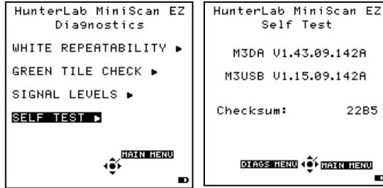
*Figure 75. Diagnostics Self-Test*
