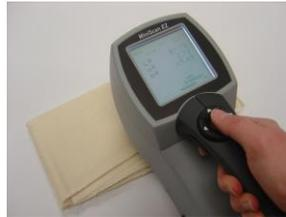
*Figure 64. Measuring Thin, Soft Materials*
