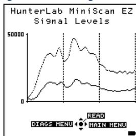
The purpose of this test is to verify that both the sample and monitor signal levels are within the correct operating range and to see channel dropouts should any occur. Press **READ** to read again. Press **DIAGS MENU** to return to the Diagnostics menu. Press **MAIN MENU** to return to the main menu.
