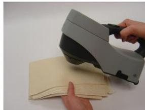
*Figure 65. Measuring Non-Opaque Samples*
