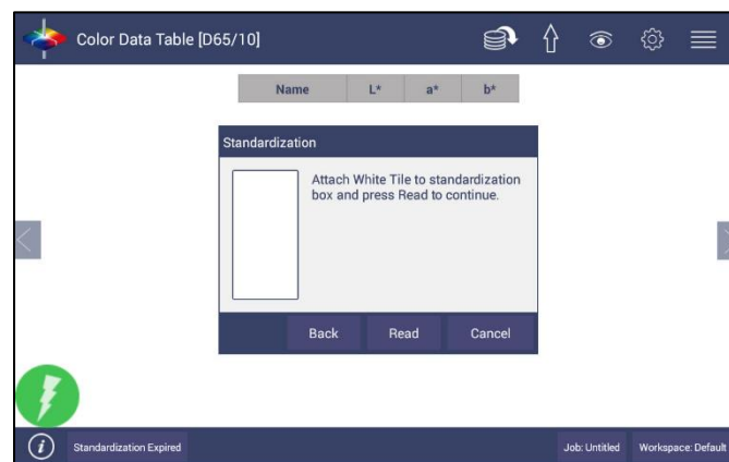
Figure 7. Read the White Tile for Top-of-Scale.
