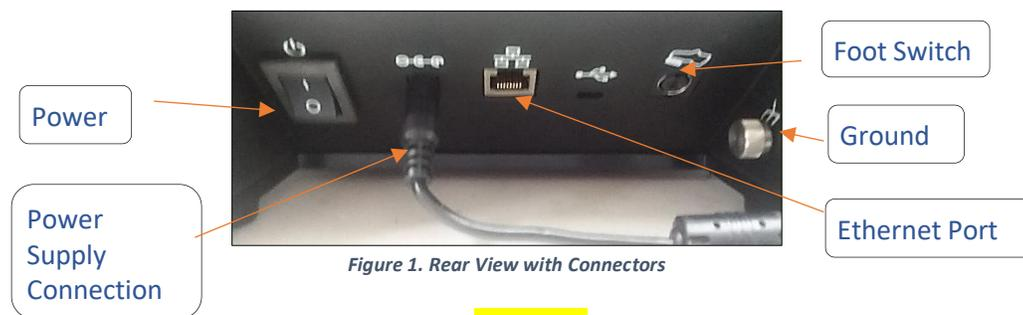
Figure 1. Rear View with Connectors
