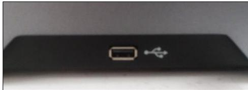
*Figure 2. USB Port on Front of Instrument*
