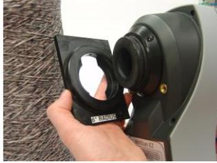
*Figure 82. Inserting the Nose Cone Adapter*
