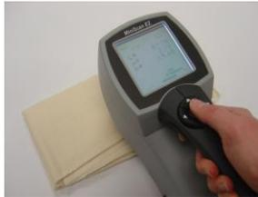
*Figure 64. Measuring Thin, Soft Materials*
