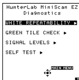
Choose the desired function by scrolling using the up and down arrow buttons until it is highlighted and then pressing the right arrow button. The various functions perform as described below.
