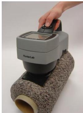
*Figure 83. Using the Nose Cone Adapter*
