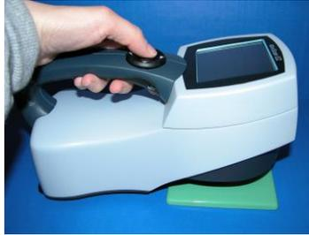
Figure 24. Reading a Standard or Sample
