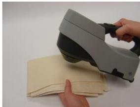
*Figure 65. Measuring Non-Opaque Samples*
