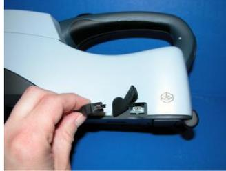
*Figure 8. Connecting the USB Cable*
