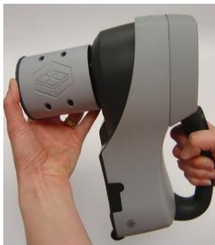
Figure 18. Reading the Calibration Cylinder
