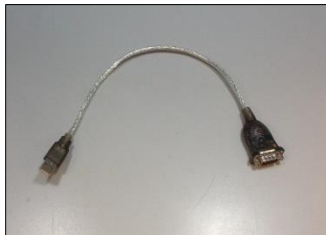
Figure 136. RS-232 to USB converter for connection via USB port
