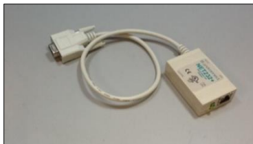
Figure 135. Ethernet to RS-232 converter for Connection via Serial port
